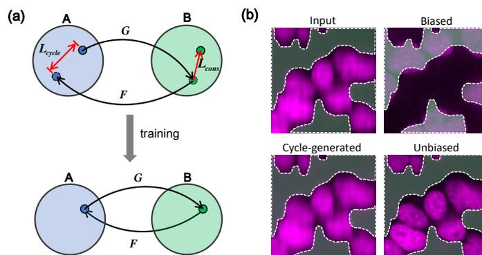
**Fig. 1.** Schematic of c<sup>2</sup>GAN. (a) *A* and *B* represent the source domain and the target domain, respectively. A forward GAN (*G*) and a backward GAN (*F*) are simultaneously trained to establish a pair of reciprocal mappings. The cycle-consistency loss ( $L_{cycle}$ ) and structural loss ( $L_{cons}$ ) are enforced to guarantee cycle consistency and high fidelity, respectively. (b) The GANs are likely to converge to biased mappings without the structural loss.
